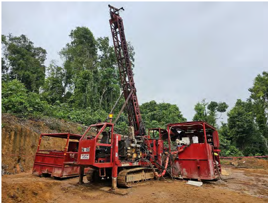
Figure 10.1: Sandvik 710 Diamond Drill Rig at the Oko West Project
