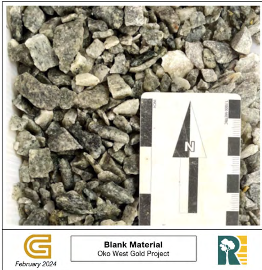
Figure 11.8: Blank Used by Company as Quality Control Sample – Oko West Gold Project
