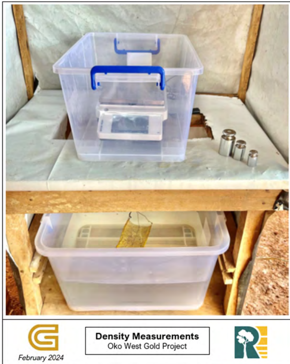
Figure 11.6: Density Measurements Balance Setup
